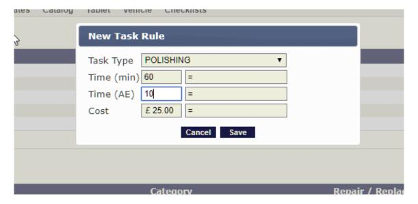
Then click save to create the new line or save the changes to the existing rule. The fields with the "=" - sign are formula fields to calculate the data when the default values are adjusted by applying the job.
