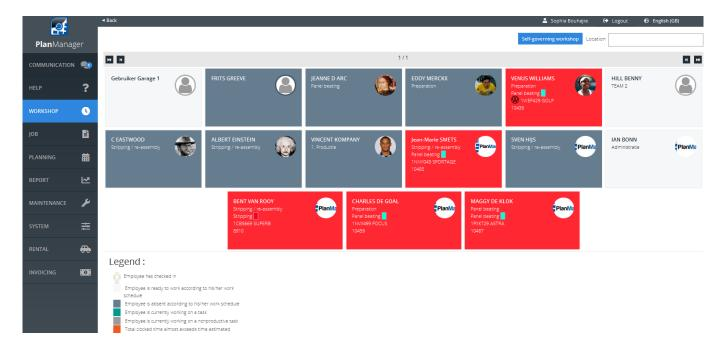
Each employee has its own field on the main screen of the ATR. If an employee wants to use the system, he must register on his block. On the screen which is then displayed he can find the current tasks and the jobs he can work on. If using the planning, these tasks will also display here.
