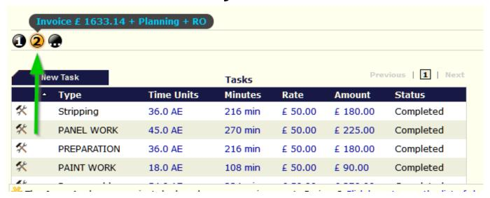
The cost column displays the cost of the activities performed. The labor cost per hour is multiplied by the hours worked by employees. In this column are also the ordered parts and the cost of the paint that was weighed shown on the paint weighing scale.
